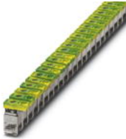
Connection terminal block, Connection method Screw connection, Load current : 125 A, Cross section: 2.5 mm 2 - 35 mm 2 , Width: 14.3 mm, Color: green-yellow
