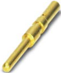
Crimp contact, diameter 1 mm, for all 3 to 5-pos. contact inserts, crimp range from 0.08 mm 2 - 0.34 mm 2 .
