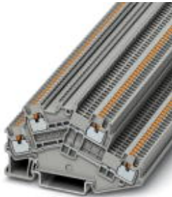
Double-level terminal block, Cross section: 0.14 mm 2 - 1.5 mm 2 , AWG: 26 - 14, Connection type: Push-in connection, Width: 3.5 mm, Color: gray, Mounting type: NS 35/7,5, NS 35/15
