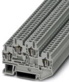
Double-level spring-cage terminal block, Cross section: 0.08 mm 2 - 4 mm 2 , AWG: 28 - 12, Connection type: Spring-cage connection, Width: 5.2 mm, Color: gray, Mounting type: NS 35/7,5, NS 35/15
