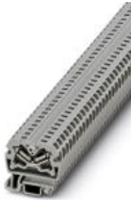
Mini feed-through terminal block, Connection method: Spring-cage connection, Cross section: 0.08 mm 2 - 4 mm 2 , AWG: 28 - 12, Width: 5.2 mm, Height: 22 mm, Color: gray, Mounting type: NS 15
