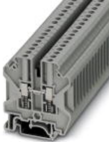
Feed-through terminal block, Connection method: Screw connection with spring support, Cross section: 0.2 mm 2 - 6 mm 2 , AWG: 24 - 10, Width: 6.2 mm, Color: gray, Mounting type: NS 35/7,5, NS 35/15, NS 32
