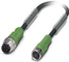
Sensor/Actuator cable, 4-position, PUR halogen-free, Black-gray RAL 7021, Plug straight M12, A-coded, on Socket straight M8, Cable length: 0.6 m
