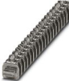
Connection terminal block, Connection method Screw connection, Load current : 41 A, Cross section: 0.5 mm 2 - 6 mm 2 , Width: 7 mm, Color: silver
