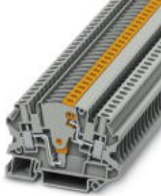
Test disconnect terminal block, Connection method: Screw connection, Cross section: 0.14 mm 2 - 6 mm 2 , AWG: 26 - 10, Width: 6.2 mm, Color: gray, Mounting type: NS 35/7,5, NS 35/15
