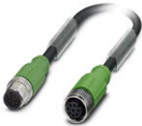
Sensor/Actuator cable, 8-position, PUR halogen-free, Black-gray RAL 7021, shielded, Plug straight M12, A-coded, on Socket straight M12, A-coded, Cable length: 1.5 m
