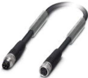
Bus system cable, INTERBUS, INTERBUS, 4-position, PUR halogen-free, Black RAL 9005, shielded, Plug straight M8, on Socket straight M8, Cable length: 10 m
