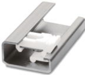
Rail adapter, snaps into NS 32 DIN rail, plastic with embedded M4 and M6 nuts, for attaching switchgear
