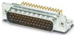
D-SUB contact insert, shell size 3, with 44 signal contacts, contact type pin, for PCB assembly, angled, fixing with 4-40 UNC thread and solder pins, for panel mounting frame VS-25-...
