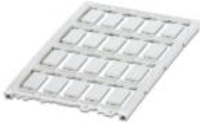
Snap-in markers, Sheet, white, Unlabeled, Can be labeled with: BLUEMARK CLED, BLUEMARK LED, Plotter, Mounting type: Snapped into marker carrier, Lettering field: 17.5 x 9 mm
