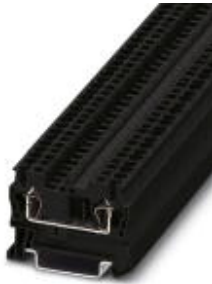
Feed-through terminal block, Connection method: Spring-cage connection, Cross section: 0.08 mm 2 - 4 mm 2 , AWG: 28 - 12, Width: 5.2 mm, Color: black, Mounting type: NS 35/7,5, NS 35/15
