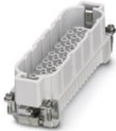
HEAVYCON male insert, D64 series, 64-pos., crimp connection. PE connection using tension sleeve technology.
