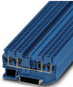
Feed-through terminal block, Connection method: Spring-cage connection, Cross section: 0.08 mm 2 - 4 mm 2 , AWG: 28 - 12, Width: 5.2 mm, Color: blue, Mounting type: NS 35/7,5, NS 35/15
