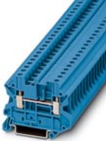
Feed-through terminal block, Connection method: Screw connection, Cross section: 0.14 mm 2 - 6 mm 2 , AWG: 26 - 10, Width: 6.2 mm, Color: blue, Mounting type: NS 35/7,5, NS 35/15
