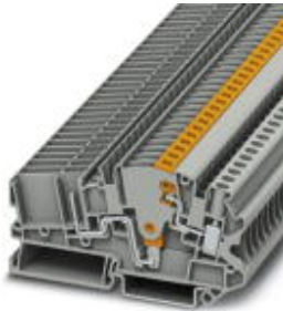
Test disconnect terminal block, Connection method: Screw/plug-in connection, Cross section: 0.14 mm 2 - 6 mm 2 , AWG: 26 - 10, Width: 6.2 mm, Color: gray, Mounting type: NS 35/7,5, NS 35/15
