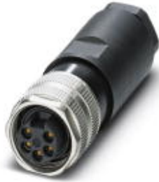
Sensor/actuator connector, female, straight, 5-pos., 7/8", screw connection, metal knurl, cable screw connection Pg13
