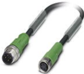
Sensor/Actuator cable, 4-position, PUR halogen-free, Black-gray RAL 7021, Plug straight M12, A-coded, on Socket straight M8, Cable length: 0.3 m
