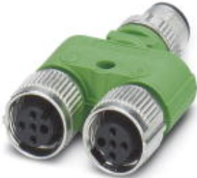
Y-distributor, 3-pos. +PE, straight plug M12 SPEEDCON on 2 x straight socket M12 SPEEDCON, PIN 2+4, bridged
