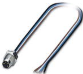
Sensor/actuator flush-type plug, 4-pos., M8, rear/screw mounting, with M8 thread, with 0.5 m TPE litz wire, 4 x 0.25 mm 2
