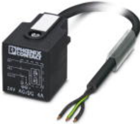
Sensor/Actuator cable, 3-position, PUR/PVC, Black RAL 9005, Free cable end, on Valve connector A, with 1 LED, Cable length: 3 m
