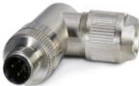
Bus system connector, PROFINET CAT5, PROFINET CAT5e, 4-position, shielded, Plug angled M12, D-coded, Insulation displacement connection, Knurl material: Nickel-plated brass, External cable diameter 4 mm ... 8 mm
