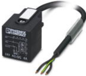
Sensor/Actuator cable, 3-position, PUR halogen-free, Black-gray RAL 7021, Free cable end, on Valve connector A, with 1 LED, connected with Z diode, Cable length: 10 m
