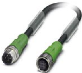
Sensor/Actuator cable, 4-position, PUR, Black-gray RAL 7021, Plug straight M12, A-coded, on Socket straight M12, A-coded, Cable length: 0.3 m
