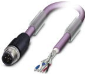
Bus system cable, CANopen ® , DeviceNet ™ , CANopen ® /DeviceNet ™ , 5-position, PUR halogen-free, Violet, RAL 4001, shielded, Plug straight M12, A-coded, on Free cable end, Cable length: 2 m
