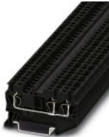
Feed-through terminal block, Connection method: Spring-cage connection, Cross section: 0.08 mm 2 - 4 mm 2 , AWG: 28 - 12, Width: 5.2 mm, Color: black, Mounting type: NS 35/7,5, NS 35/15
