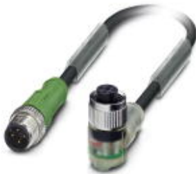
Sensor/Actuator cable, 4-position, PUR halogen-free, Black-gray RAL 7021, Plug straight M12, A-coded, on Socket angled M12, A-coded, with 3 LEDs, Cable length: 3 m
