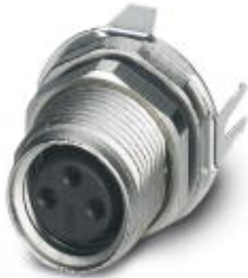
Sensor/actuator flush-type connector, socket, 3-pos. M8, rear/screw mounting with M10 fastening thread, with straight solder connection
