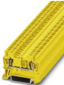
Feed-through terminal block, Connection method: Spring-cage connection, Cross section: 0.08 mm 2 - 4 mm 2 , AWG: 28 - 12, Width: 5.2 mm, Color: yellow, Mounting type: NS 35/7,5, NS 35/15
