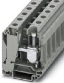
Feed-through terminal block, Connection method: Screw connection, Load current : 125 A, Cross section: 10 mm 2 - 35 mm 2 , AWG 8 - 2, Width: 15.1 mm, Color: gray
