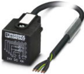
Sensor/Actuator cable, 5-position, PUR halogen-free, Black RAL 9005, Free cable end, on Valve connector AD (pressure switch), with 2 LEDs, Cable length: 1.5 m
