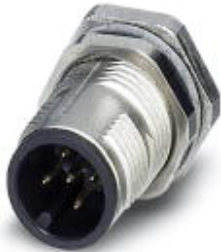
Sensor/actuator flush-type plug, 5-pos., M12 SPEEDCON, A-coded, rear/screw mounting with M12 thread, with straight solder connection
