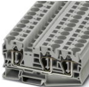
Feed-through terminal block, Connection method: Spring-cage connection, Cross section: 0.2 mm 2 - 25 mm 2 , AWG: 24 - 4, Width: 12.2 mm, Color: gray, Mounting type: NS 35/15, NS 35/7,5
