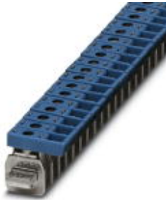
Connection terminal block, Connection method: Screw connection, Cross section: 0.5 mm 2 - 6 mm 2 , AWG: 20 - 10, Width: 7 mm, Height: 23.6 mm, Color: blue, Mounting type: Neutral busbar
