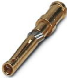
Turned 1.6 crimp contact, individual female contact, core diameter 1.5 mm 2 , gold-plated
