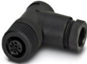
Sensor/actuator connector, female, angled, 5-pos., M12, A-coded, screw connection, plastic knurl, cable screw connection Pg9
