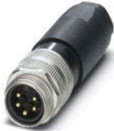
Sensor/actuator connector, male, straight, 5-pos., 7-8", screw connection, metal knurl, cable screw connection Pg13
