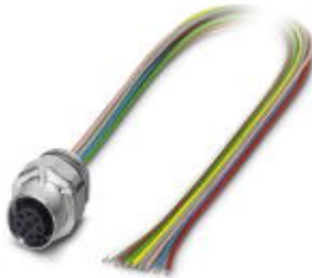
Sensor/Actuator flush-type socket, 8-pos., M12-SPEEDCON, A-coded, front/screw mounting with M16 thread, can be positioned, with 0.5 m TPE litz wire, 8 x 0.25 mm 2
