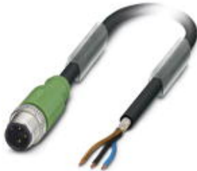
Sensor/Actuator cable, 3-position, PUR halogen-free, Black-gray RAL 7021, shielded, Plug straight M12, A-coded, on Free cable end, Cable length: 1.5 m
