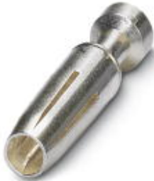
Turned 2.5 crimp contact, individual female contact, core diameter 2.5 mm 2 , silver-plated
