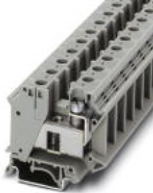
Installation terminal block, Screw connection, Cross section: 0.75 mm 2 - 35 mm 2 , AWG: 18 - 2, Width: 15.2 mm, Color: gray, Mounting type: NS 35/7,5, NS 35/15
