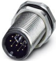
Sensor/actuator flush-type plug, 12-pos., M12, rear/screw mounting with M12 thread, with straight solder connection
