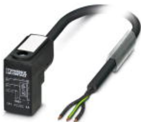
Sensor/Actuator cable, 3-position, PUR halogen-free, Black-gray RAL 7021, Free cable end, on Valve connector C (8 mm), with 1 LED, connected with Z diode, Cable length: 1.5 m
