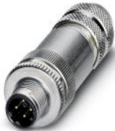
Bus system connector, male, straight, 4-pos., M12, shielded, D-coded, screw connection, metal knurl, cable screw connection Pg9
