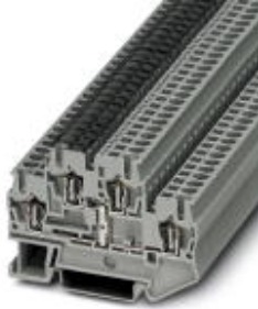
Feed-through terminal block, Cross section: 0.08 mm 2 - 4 mm 2 , AWG: 28 - 12, Connection type: Spring-cage connection, Width: 5.2 mm, Color: gray, Mounting type: NS 35/7,5, NS 35/15
