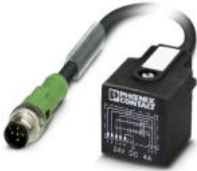
Sensor/Actuator cable, 5-position, PUR halogen-free, Black RAL 9005, Plug straight M12 SPEEDCON, A-coded, on Valve connector AD (pressure switch), with 2 LEDs, Cable length: 1.5 m
