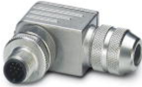
Connector, Universal, 12-position, shielded, Plug angled M12, A-coded, Solder connection, Knurl material: Zinc die-cast, nickel-plated, Cable gland Pg9, External cable diameter 6 mm ... 8 mm
